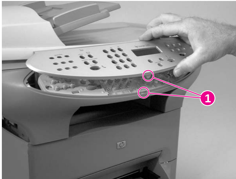
Figure 5-23. Reinstall the control-panel bezel (1 of 2)
