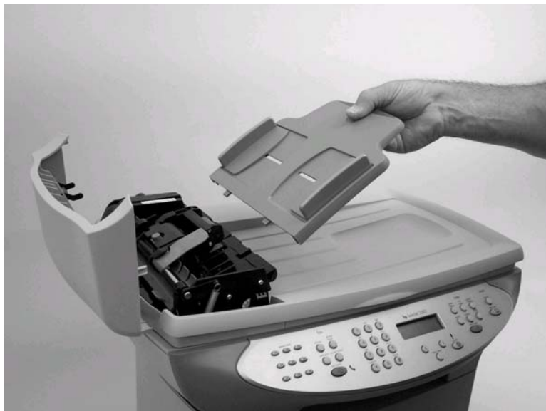
Figure 5-12. Remove the ADF pickup-roller assembly (1 of 5)
