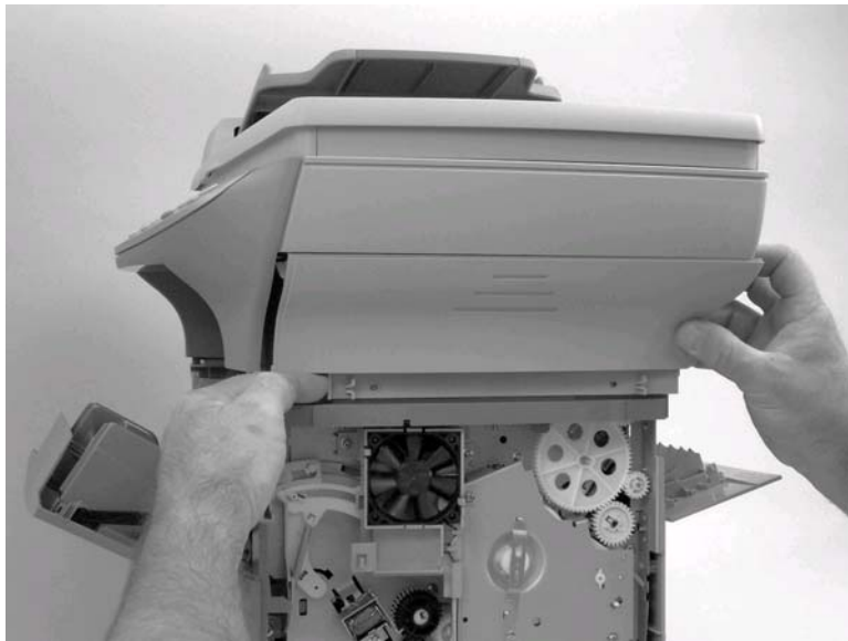
Figure 5-8. Remove the scanner right-side cover (2 of 2)
