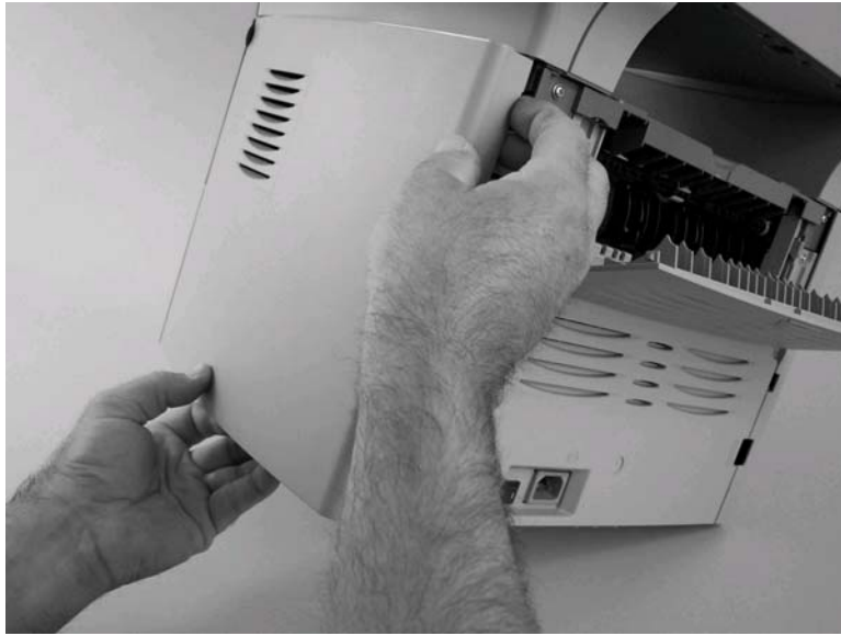
Figure 5-5. Remove the printer right-side cover (2 of 3)
