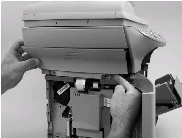
Figure 5-10. Remove the left-side scanner cover (2 of 2)
