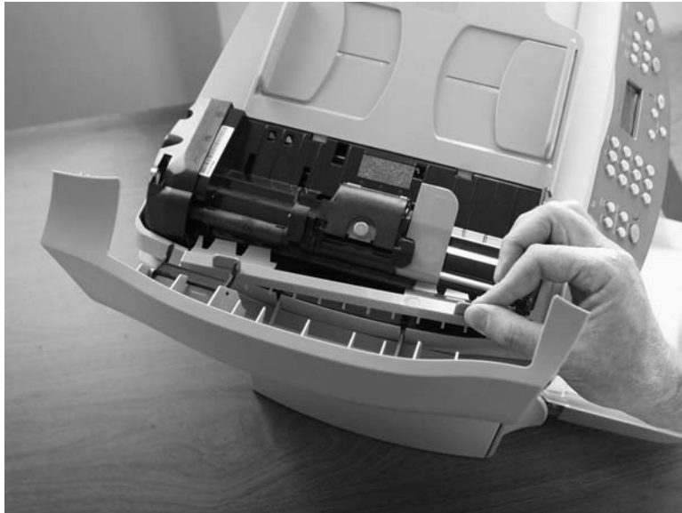
Figure 5-17. Remove the ADF document-feed guide/cleanout comb
